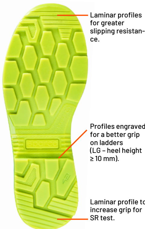
Dual density PU OUTSOLE with special design of the lugs which guarantee maximum grip in all flexion conditions. SR + FO + LG
